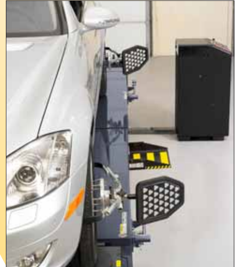
Lightweight durable targets are easy to install.
