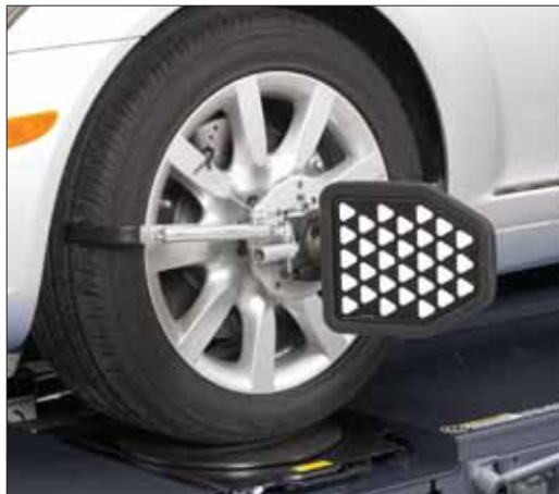
Targets have no electronics to damage if dropped.
