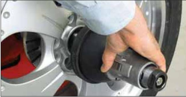
The optional AutoClamp feature saves time and effort. The clamp adaptor is positioned and tightened automatically. There are no time-consuming shaft threads to take-up and no additional wing nut tightening required.
