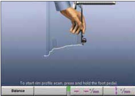
The inner Dataset arm will trace the exact wheel contour and store the scanned distances and diameters for all available tape weight locations selected by the operator. Rim Scan also offers the benefits of Automatic Weight Positioning to increase the capability to single spin balance with SmartWeight technology.
