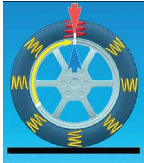
*Offering the same service as new car vehicle manufacturers, the GSP9700 matches the stiffest area or high spot on the tire with the lowest spot on the rim to cancel vibration caused by radial force variation and provide the smoothest possible ride.*
