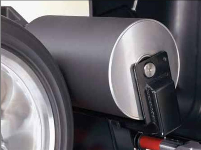
The exclusive Road Force Measurement® system applies up to 1,400 pounds (635 kg) against the tire. The loaded roller detects non-balance, radial-force-related vibrations caused by eccentricity and constructional variation of the tire and wheel. Unlike non-contact measurement, the roller samples the entire footprint of the tire including the sidewall's contribution to ride quality.
