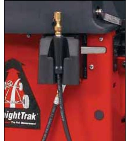
*GSP9700's Inflation Station\* provides proper inflation pressure and automatic prompting for the operator to ensure accurate testing and customer satisfaction.*
