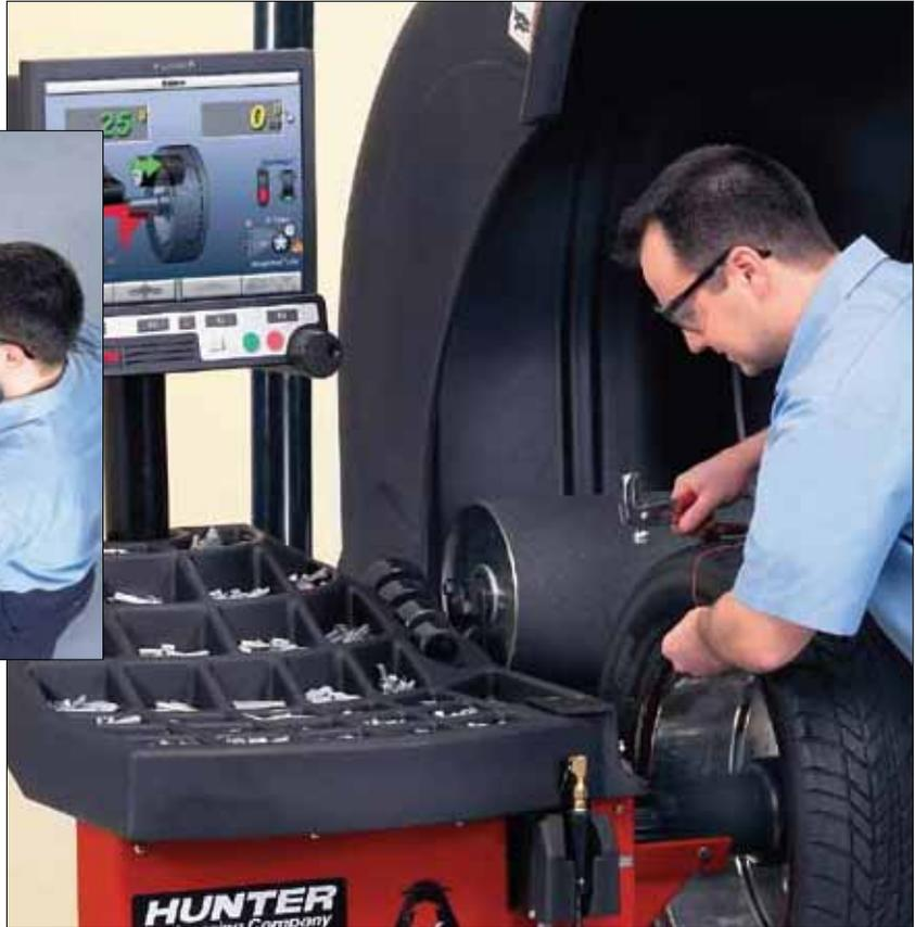
Hunter's patented ForceMatching® feature cancels the stiffest point of tire radial force variation with the low spot on the rim. This helps eliminate vibration by minimizing the effects of radial force variation and rim runout.
