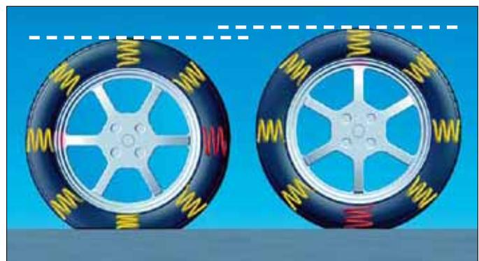
*Lack of tire uniformity is a common and often hidden source of vibration. As a tire rolls, it flexes as if it were made of springs. Vibration results when tire stiffness is not uniform.*
