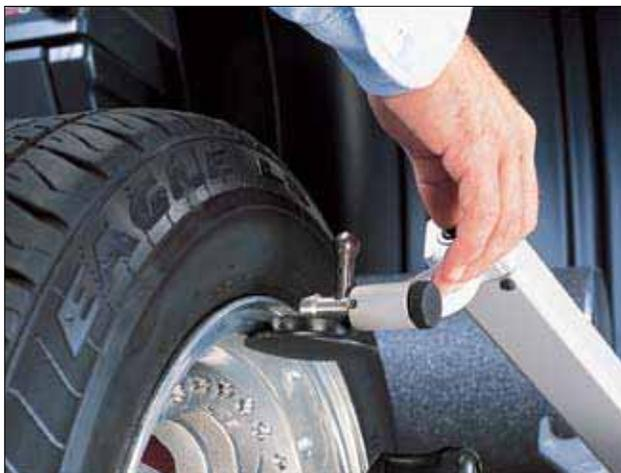
*Rim runout can be measured without removing the tire...*
