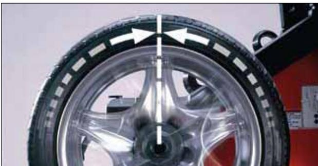
Servo Stop automatically rotates and positions wheel to each desired weight location (TDC or BDC) with the touch of a button or by simply pushing the wheel.
